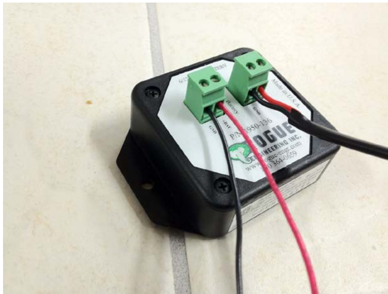
Insert the straight ends of the wires into the charge conditioner and tighten the “jaws” The Red wire goes into “+BAT”
