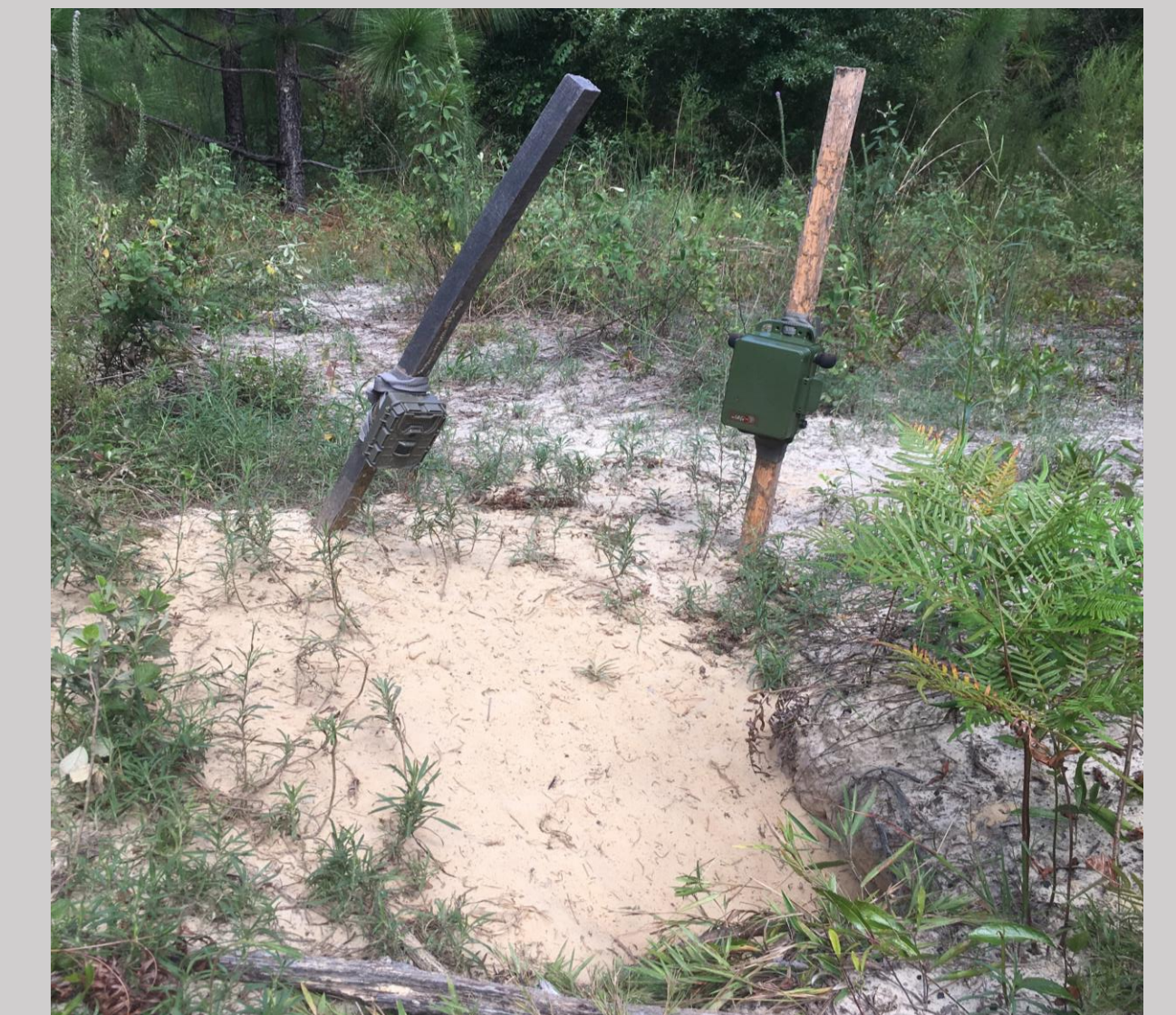
This image shows a Bushnell game camera and Wildlife Acoustics SM4 audio recorder, deployed at the burrow of a tracked resident female.
