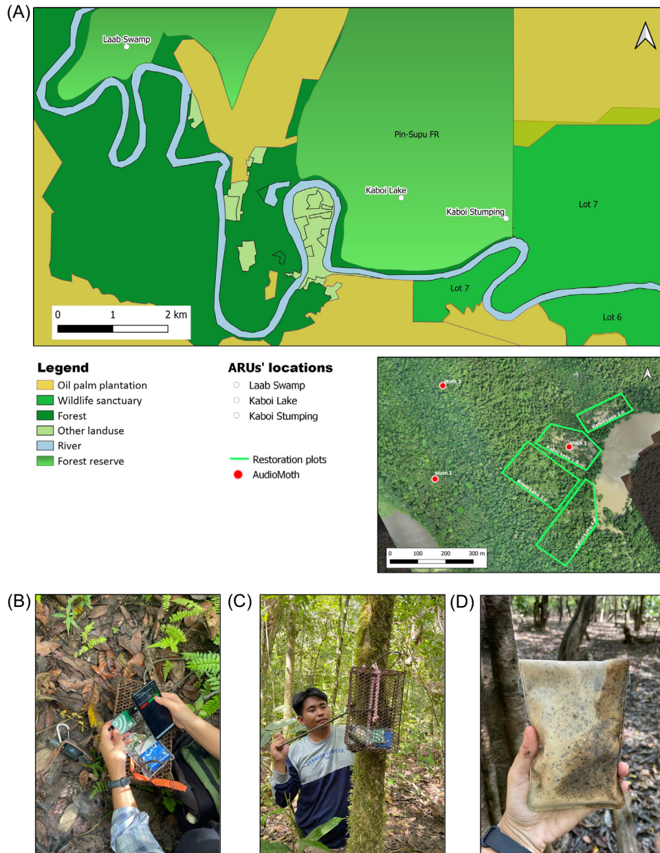
Figure 3. Set-up and deployment of autonomous recording unit (ARU) in Sabah, Malaysia. (A) Map Kinabatangan floodplain. Inset photo illustrates AudioMoths (red) deployed in and near forest restoration plots (green lines) at Kaboi Lake. (B) Programming and setting up ARU. (C) Positioning ARU with battery pack in waterproof casing and protective wire cage. (D) ARU waterproof case after 10 days submerged in floodwater.
