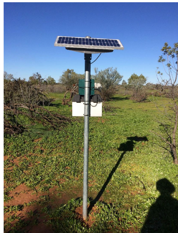
Figure 3. The acoustic monitoring station from Thompson Creek in Sturt National Park. The black panel at the top of the station is the solar panel, the green box is the Wildlife Acoustics Songmeter SM2+ and the white box is a weatherproof case that holds the deep cycle battery and charge regulator.
