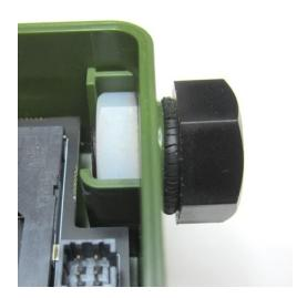
If you see degradation or are worried about this in the future, we will replace your O-ring free of charge. The replacement O-ring is red/orange in color, made of silicone and will not degrade. A few weeks ago, we switched our manufacturing to the new silicone O-ring. If your O-ring is red/orange as shown below, you are not affected by this bulletin.
