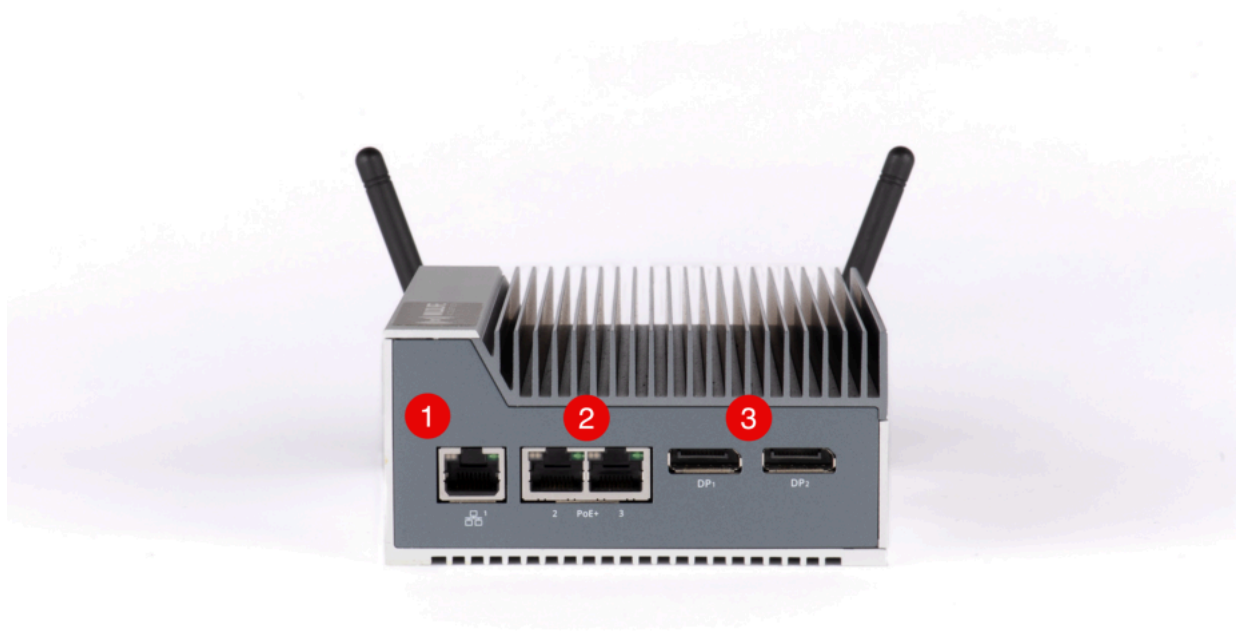
Figure 1. SMART Controller Connectivity: Ethernet and DisplayPort
